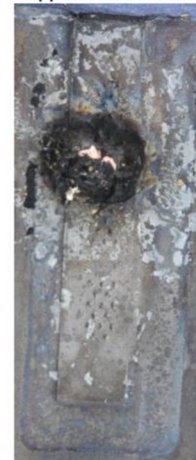
Negative Electrode Opposite Positive Tab
