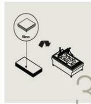
The parts are cut by a CNC mill using locally-bought material. This is 18mm plywood, in the standard sheet size of 2440mm x 1220mm (8' x 4').
