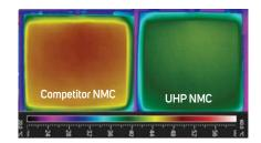
UHP Cell creates less heat than standard NMC cells, allowing for more vigorous operations
